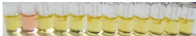
Fig. 7 Color changes of compound 1 (20 \mu\text{M} ) on addition of different metal ions (80 \mu\text{M} ) in ethanol/aqueous tris buffer (9:1, v/v) of pH 9.17. From left to right: blank, \text{Hg}^{2+} , \text{Zn}^{2+} , \text{Cd}^{2+} , \text{Mn}^{2+} , \text{Co}^{2+} , \text{Ni}^{2+} , \text{Cr}^{3+} , \text{Fe}^{3+} , \text{Cu}^{2+} , \text{Pb}^{2+} , \text{Ag}^+
